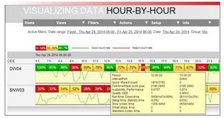
Hour-By-Hour - The display provides a color coded timeline by hour and part produced, with 'hover' details for each timeline segment. There is a choice of data aspects to report upon (i.e. Good count, OEE, Small stops, etc).
