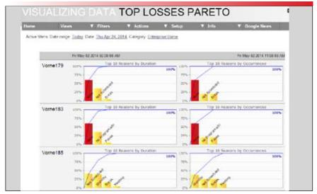
Top Losses Pareto - Compare top losses across multiple lines, including setup and standby.
