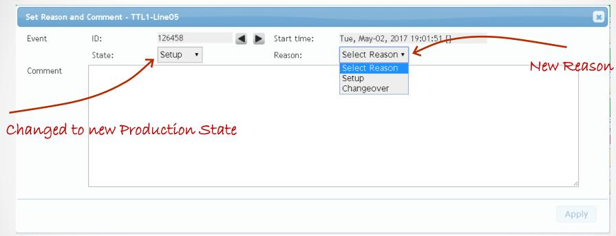
Changing production state causes the OEE calculations to change and all related values must be recalculated. We cannot change the state in the Vorne, but if we are changing the state of the current event, we can split the event so the requested state is present going forward. But it is important to recognize that the Vorne and OEEAlert will now have different data and as a result, different OEE values.
